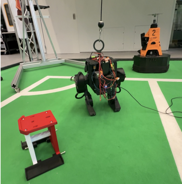
Fig. 5: Image Highlighting the Test Setup, including the stand for the robot (left) and the hook used to attach to the tether.
